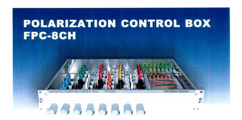
Our new Polarization Control Box, FPC-8CH, is an 18½" rack-mountable unit consisting of eight separate manual polarization controllers. Individual 3-stage rotary knobs provide independent control for any desired state-of-polarization. This modular structure is suitable for DWDM applications and enables quick, easy transport of large numbers of polarization controllers between laboratories.
